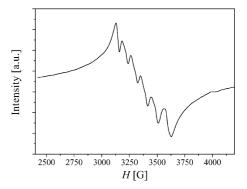
Figure 4. EPR spectrum recorded at room temperature for sample I [1.20% Mn from Mn(acac)<sub>3</sub> precursor].
