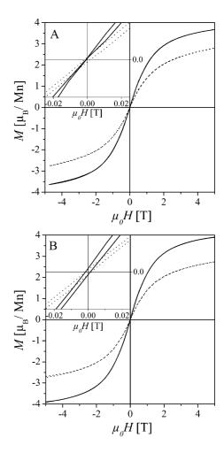
Figure 6. Hysteresis loops at T=2 K for (A) samples from Mn(ac)<sub>2</sub> with 1.39% Mn (solid line) and 4.38% Mn (dotted line) and (B) samples from Mn(acac)<sub>3</sub> with 1.20% Mn (solid line) and 4.85% Mn (dotted line).
