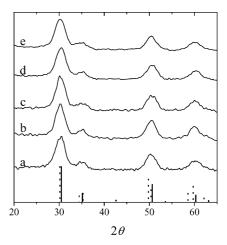
Figure 1. XRD patterns of (a) undoped zirconia; (b) zirconia doped with 1.39% of Mn(ac)<sub>2</sub>; (c) zirconia doped with 1.20% of Mn(acac)<sub>3</sub>; (d) zirconia doped with 4.38% of Mn(ac)<sub>2</sub>; (e) zirconia doped with 4.85% of Mn(acac)<sub>3</sub>. Theoretical reflection of cubic phase (vertical full line) and tetragonal phase (vertical dotted line) are specified.
