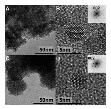
Figure 2. (A) TEM overview image showing an agglomeration of 4.38% Mn-ZrO<sub>2</sub> doped particles synthesized from Mn(ac)<sub>2</sub>; (B) corresponding HRTEM image of a particle in the [110] orientation with the respective power spectrum (inset); (C) TEM image of pure zirconia sample; (D) corresponding HRTEM picture showing a single particle in the [110] orientation and its power spectrum.
