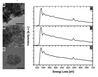
Figure 3. EELS spectra recorded from different agglomerations of 4.38% Mn-doped particles (A), (B), and (C). The TEM images show the amount of particles that have contributed to each spectrum. Scale bars correspond to 50, 10, and 10 nm for A, B, and C, respectively.
